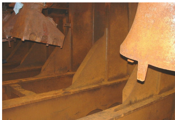
Figure 1. Marine coating degradation showing cracks and rust in water ballast tanks
